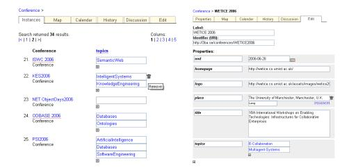
**Figure 4.** Editing of a property's values at many instances at once (left). Dynamically generated form combining different widgets based on an OWL class definition (right).
